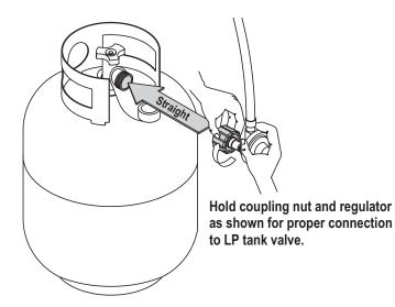
6. Turn the coupling nut clockwise and tighten to a full stop. The regulator will seal on the back-check feature in the LP tank valve, resulting in some resistance. An additional one-half to three-quarters turn is required to complete the connection. Tighten by hand only – do not use tools.
